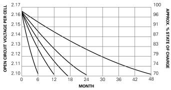
The maximum storage times before a refresh charge is required and recommended open circuit voltage audit intervals are:
