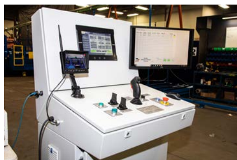
Automation control terminal for BBE-FA (including options)
