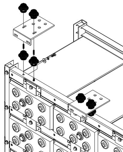
TERMINAL PLATE INSTALLATION DETAIL
