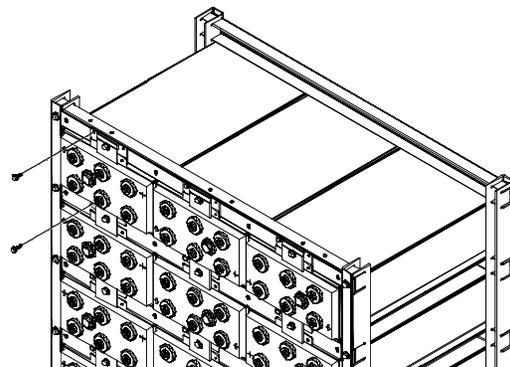
INSTALL BONDING SCREWS
