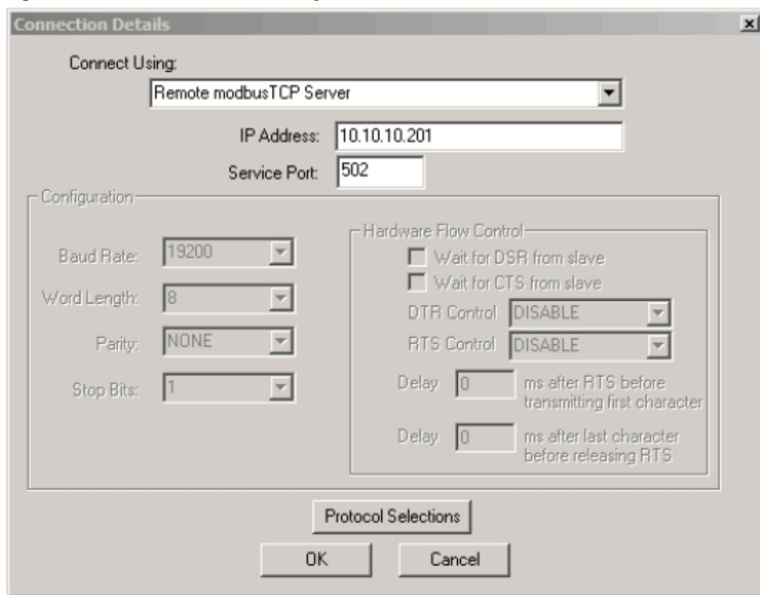
Once a connection is made, data is polled automatically at the given device ID, address, and length as shown.
