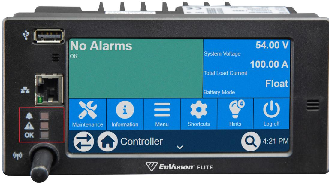
Figure 3: EnVision™ Elite Touch controller LEDs
