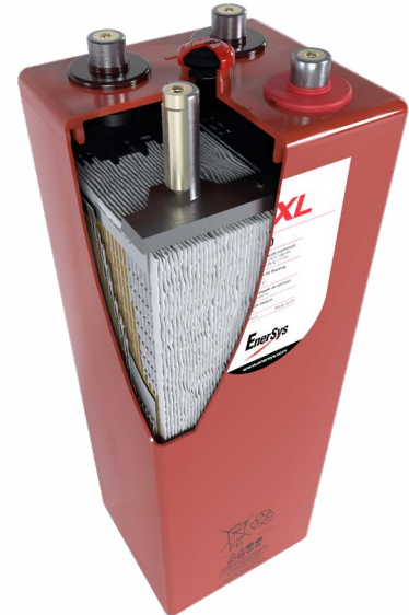
Figure 2: A detailed cutaway of a PowerSafe® SBS XL 2V Battery cell with TPPL technology"
