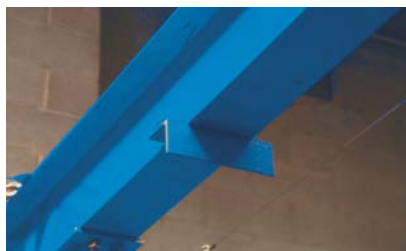
Adjustable hoist stop (Assists in precise battery positioning & prevents damage)
