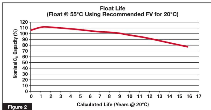
Battery life is reduced by 50% for every 10°C/18°F increase in temperature (see figure 3). Float voltage compensation reduces the charging current as battery temperature increases and partially negates the adverse effect of high temperature.
