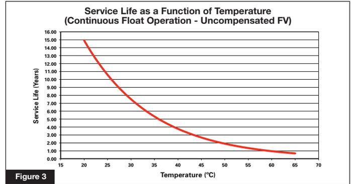
The recommended float voltage temperature compensation is:
