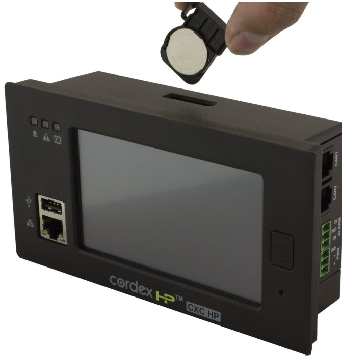
Figure 65: Controller battery replacement
