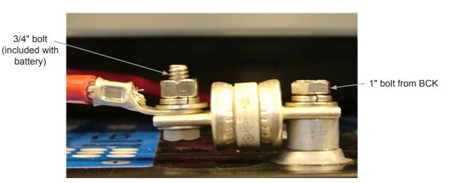
Fig. 2, Fuse Terminal Connection
