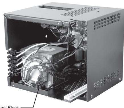
Fig. 9-2, Location of Terminal Block
