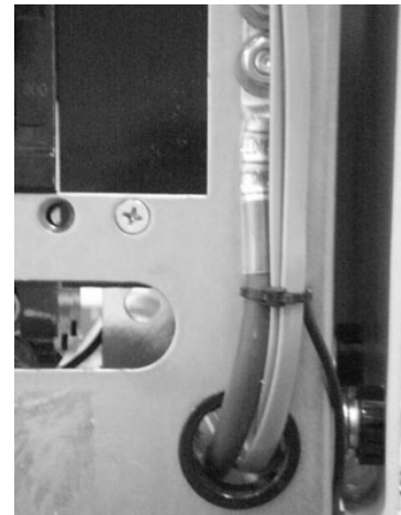
Figure 4. Temperature sensor cable routing through DCX chassis via grommet hole and up to DCX control PCB jack locations
