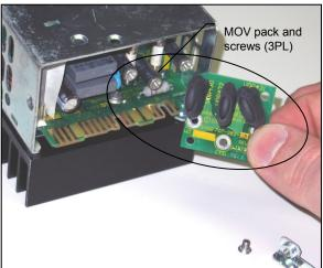
Figure 10-Showing MOV removal and replacement
