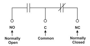
Figure 8-Showing relay connections
