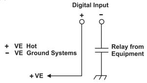
Figure 7-Showing digital input connection method
