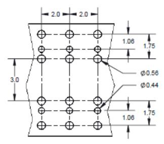
Figure 51 — Customer Connections Spacing
