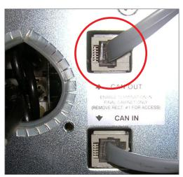
Figure 38 — CAN IN/CAN OUT Connection 4.0kW
