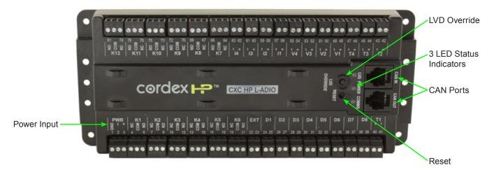
Figure 24 — L-ADIO I/O Peripheral
