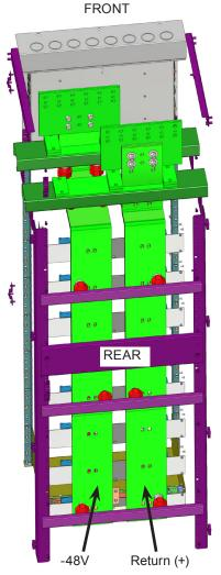
Figure 3 — Stand-alone Power Bay showing DC Charge Buses
