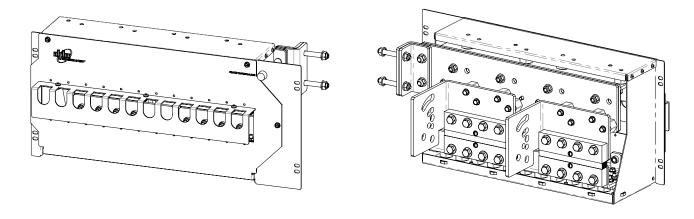
Figure 14 — 2x 6 Position High Capacity Breaker
