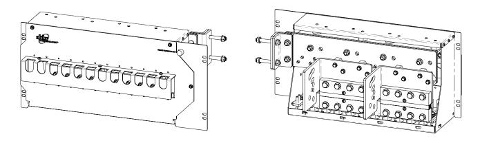
Figure 13 — 2x 5 Position High Capacity Breaker
