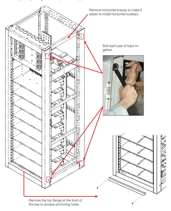
Figure 30 — Bolting Adjacent Bays Together
