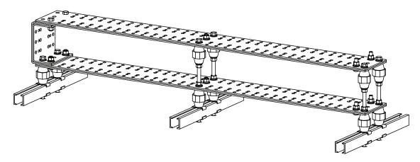
Figure 21 — External Battery Return Ground Bar (2 bars shown)
