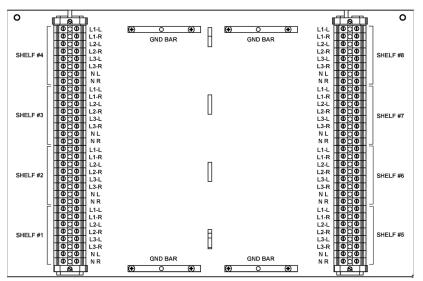
Figure 47 — Terminal Blocks for 16-feed 208/480Vac input
