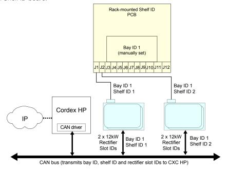
Figure 52 — Example of a Single Bay with Two Rectifier Shelves.
