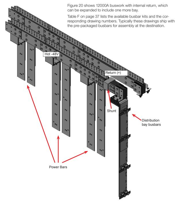
Figure 20 — Inter-bay DC Connections (Front View)
