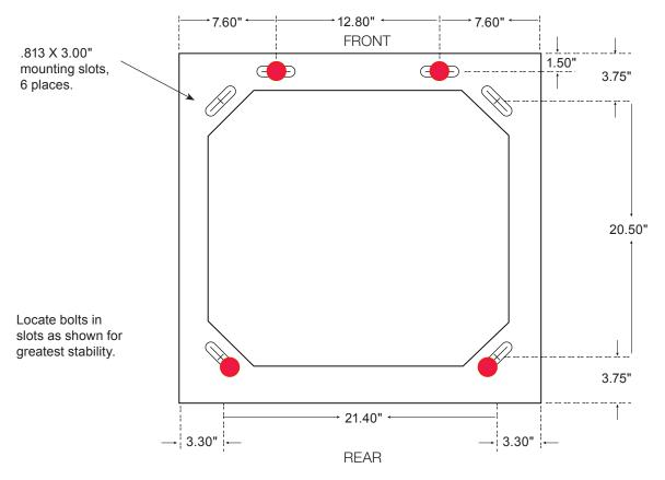
Figure 28 — Base Dimensions and Mounting Holes
