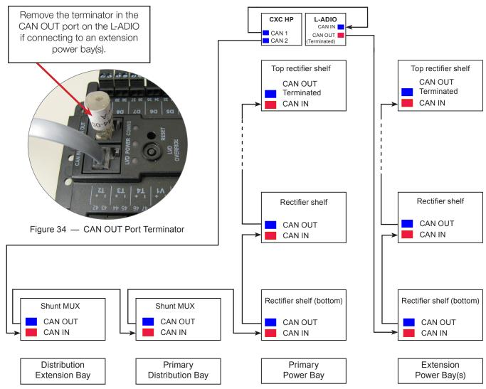
Figure 35 — Controller, CAN Bus cabling 4.0kW Power Bay
