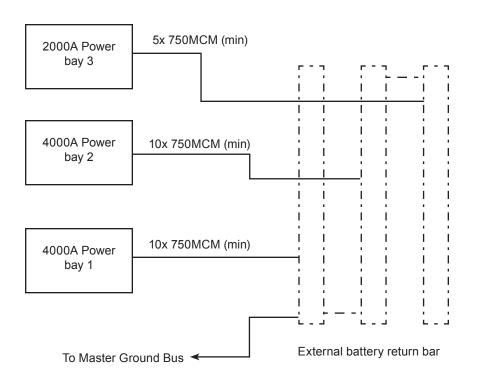
Figure 50 — External Battery Return Bar Wiring
