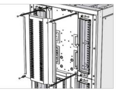
Fig. 1, BDFB front panel removal
