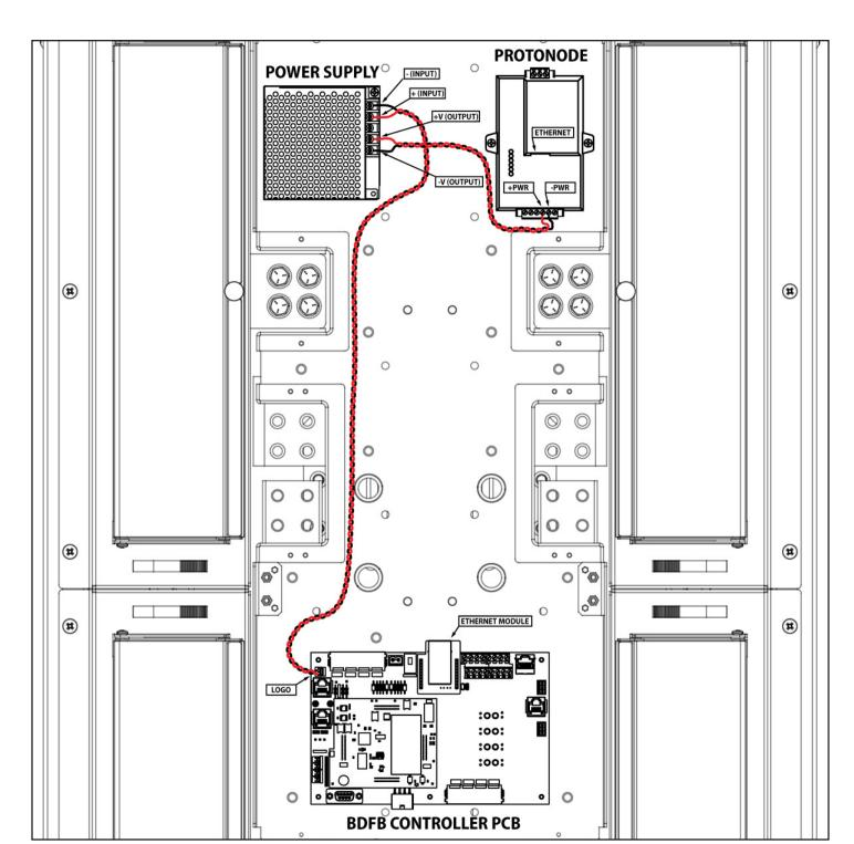
Fig. 3, Wire layout detail
