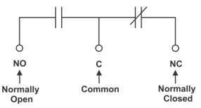
Relays can be programmed to energize or de-energize during an alarm condition (see controller software manual). When the CXCM1 reset button is pressed or power is lost, all relays de-energize.
