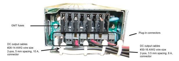
**NOTE:** Make sure the applicable fuse has been removed before unplugging the corresponding connector.
