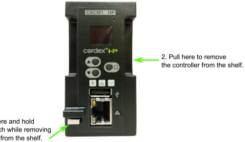
1. Push up here and hold to release latch while removing the controller from the shelf.
