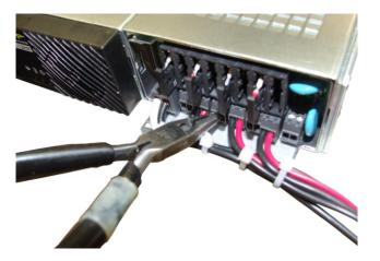
2. After the plug-in connector has been removed, attach the cables to the terminal block. Verify the polarity.
