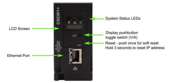
Figure 12: Cordex CXCM1+ model system controller front panel
