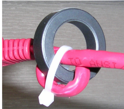
Figure 19 — Ferrite ring installed on RJ45 network cable
