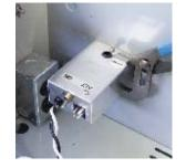
2. Hold the SPI in place using channel lock pliers while tightening nut. Torque to 130 in/lbs.
