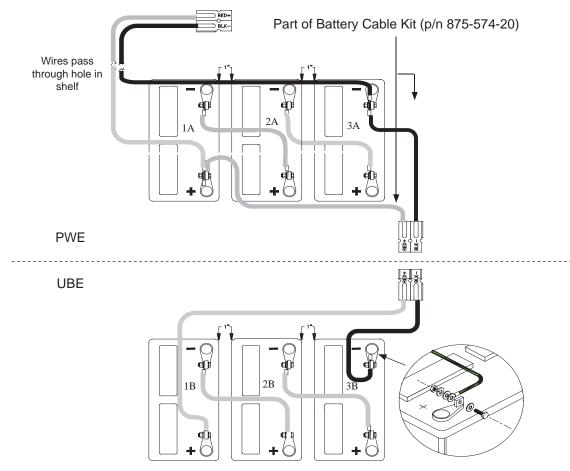
Fig. 11, Battery Wiring Diagram
