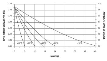
The maximum storage times before a refresh charge is required and recommended open circuit voltage audit intervals are:
