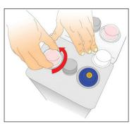
8. Fit inter-cell connectors. Torque them to 25Nm.
