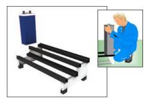
2. Install the other cells with the appropriate spacing between cells in mind.
