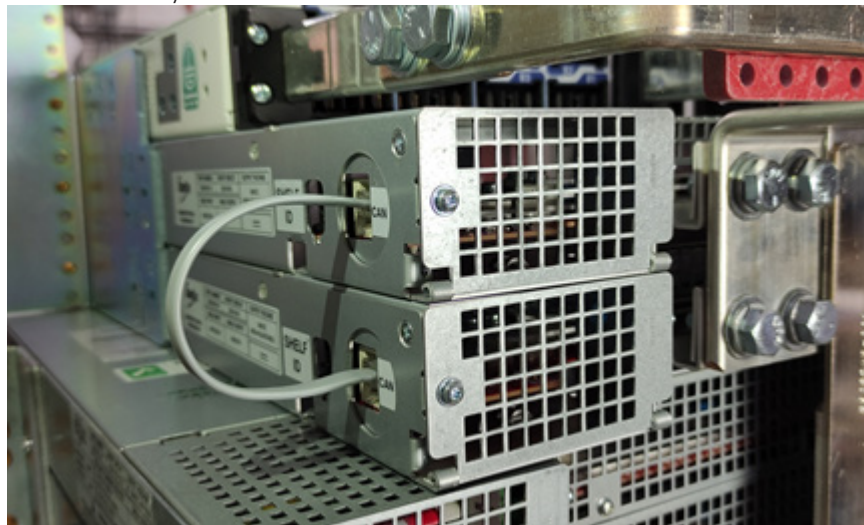
Figure 15: Inter-shelf CAN cable assembly
