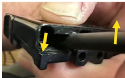
Use an insulated flathead screwdriver, push down on DC terminal spring and use leverage.
