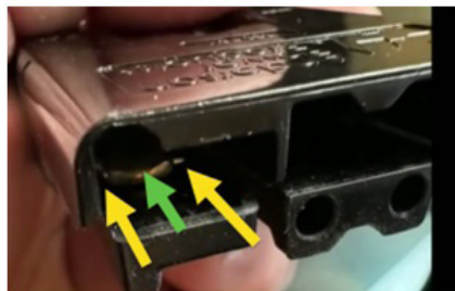
Yellow arrow: retention spring Green arrow: DC contact
